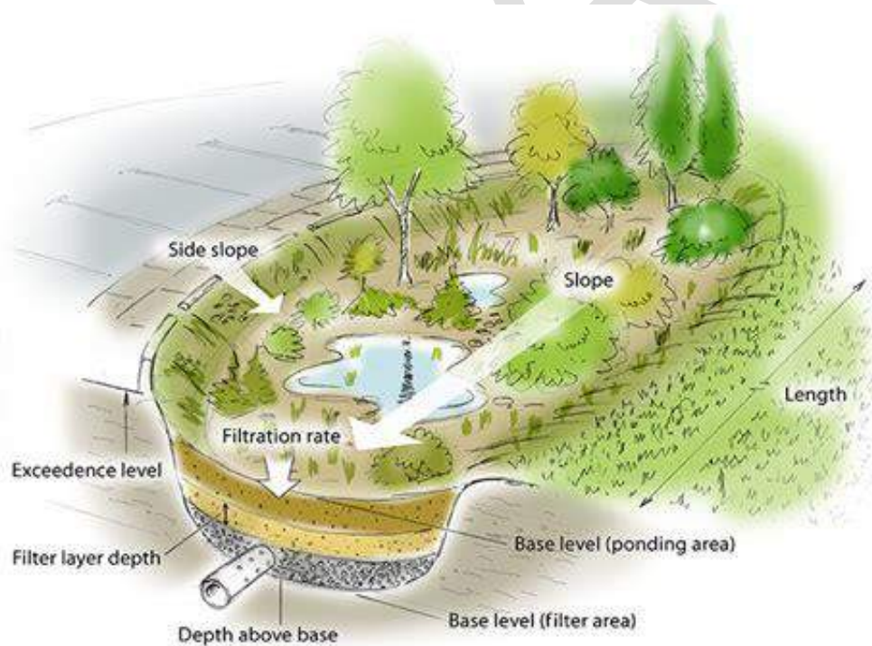
Figure 38 Diagram of stormwater bio-retention system 110 .
